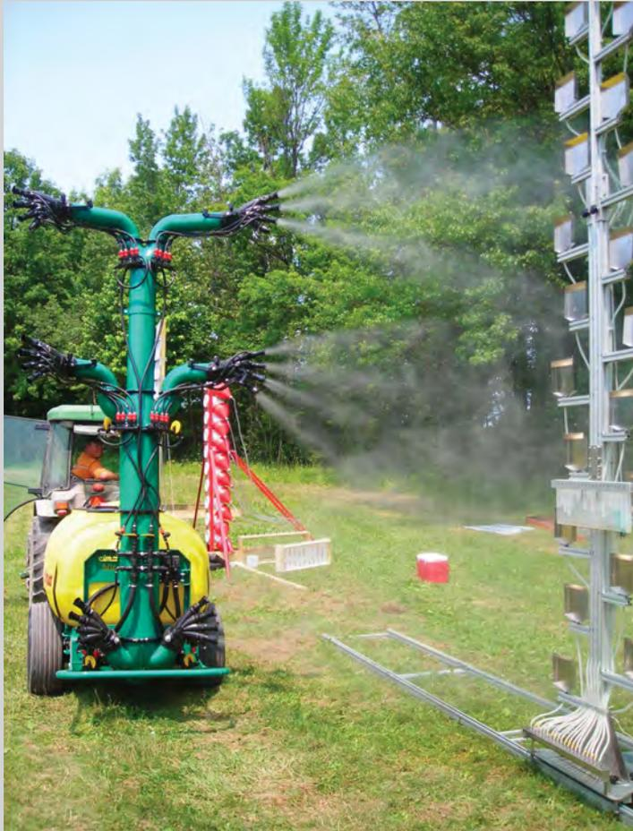
Fig. 18 – **Example** of vertical distribution pattern evaluation using a sprayer with individual outputs (Photo E. Gil, UPC Barcelona).
