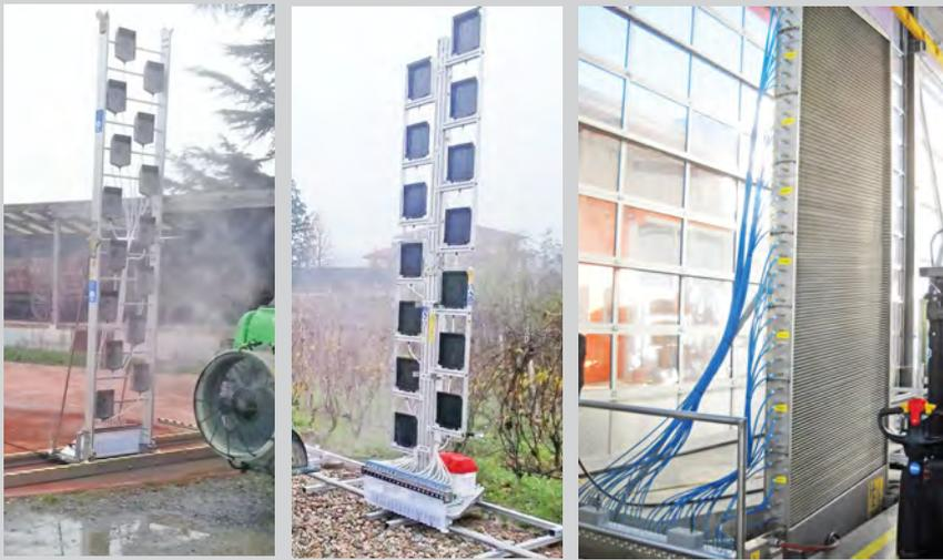
Fig. 10 – **Examples** of vertical test benches provided with discrete or continuous elements (Photo G. Oggero, DiSAFA Torino University).
