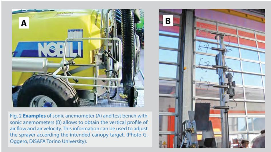
Fig. 2 **Examples** of sonic anemometer (A) and test bench with sonic anemometers (B) allows to obtain the vertical profile of air flow and air velocity. This information can be used to adjust the sprayer according the intended canopy target. (Photo G. Oggero, DiSAFA Torino University).
